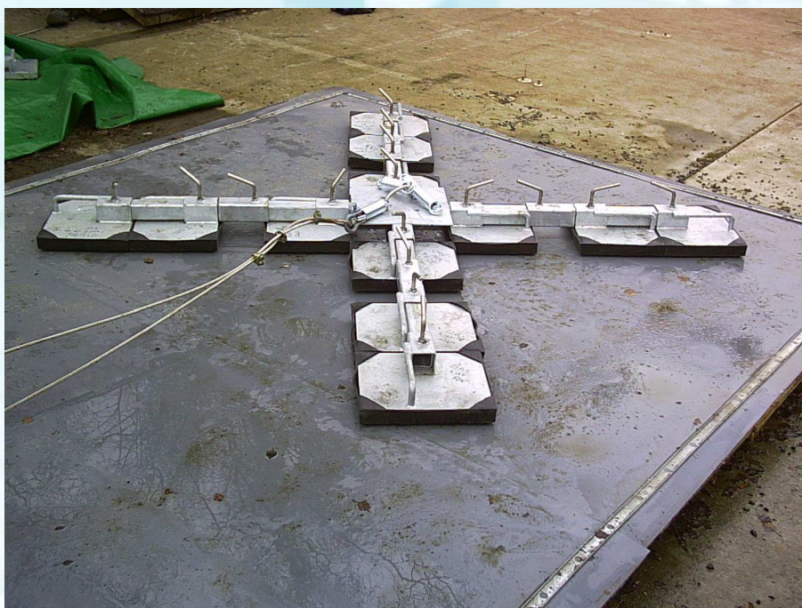
Figure 2 – Mobile Man Anchor reference “21AS Cup type” mounted on Single-ply membrane roof before testing
